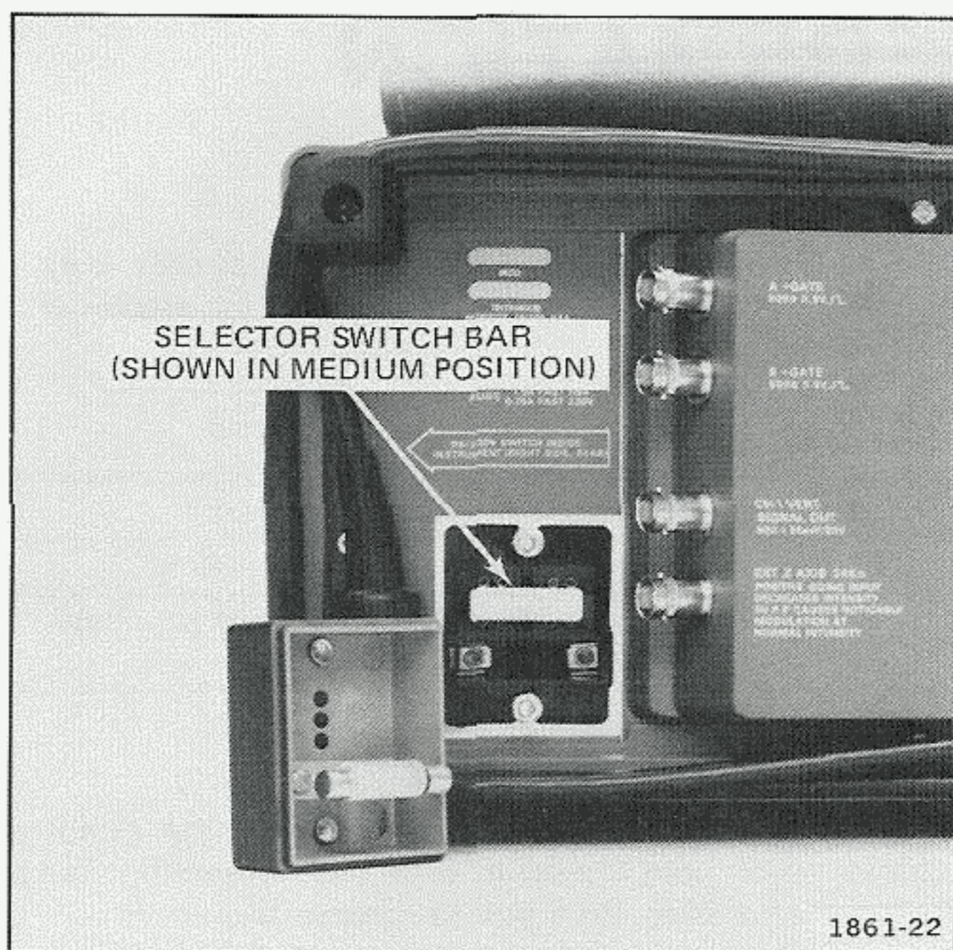
Fig. 2-1. Power supply regulating range selector.
